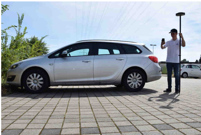
The SP80 is excellently suited for the accurate determination of position and speed, e.g., here while calibrating a parking space or vehicle dimensions
