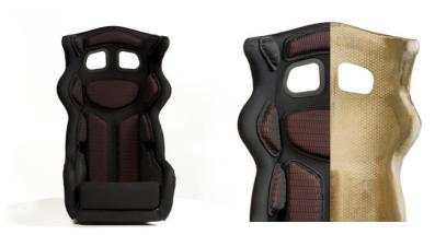
The shell structure includes a honeycomb layer that increases the rigidity of the shell, to give to drivers a better feedback of the car and allow them to sharpen the set-up. The increased stiffness guarantees that the seat will preserve the same characteristics throughout its life without any distortion, giving it a useful life of 6 years with possible extension of 2 years. Thanks to this manufacturing process, GP-RACE offers an
