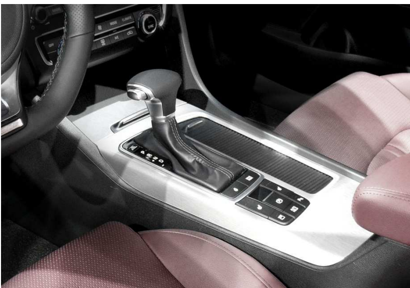
Amcor's CoolTouch™ lightweight formable aluminium on the KIA Optima 2016 gear panel cover
